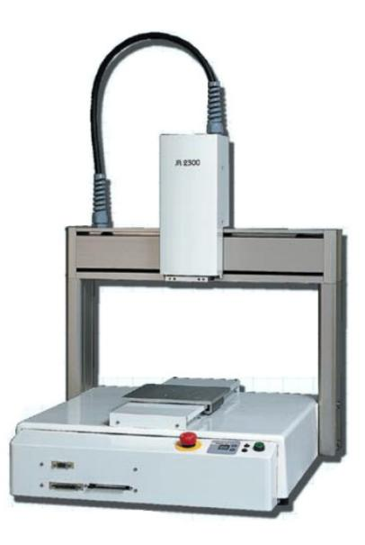
Even complex program patterns can be developed quickly using the simple point to point teach pendant. Dispense adhesive direct from syringes or optional metering valves and pressure pots. With fast indexing speeds, high accuracy and simple programming; robots are an ideal solution for most dispensing applications in a 300mm x 320mm work area. 3 or 4 axis versions available. Recommended optional light guard safety cages also available.
